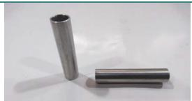
**Booms** used in Telecom Industry made of Aluminium Alloy of various lengths and diameters based on the frequency required, speciality if Diameter control in 20 microns, Circularity control in 15 microns and Perpendicularity control in 20 microns.
